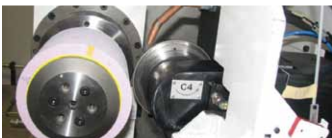
5. Machine automatically compensates changes via a dressing cycle.
