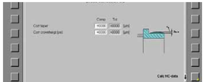
4. Input actual measured values into control. Control calculates adjustments based on measured values.
